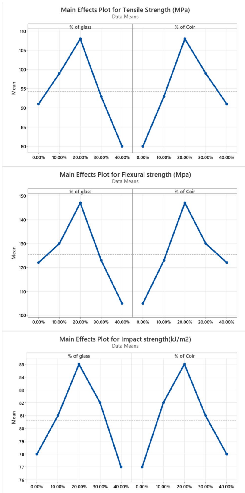
Figure 5: Main effects plots for tensile strength, flexural strength and impact strength
