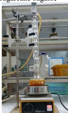
Figure 3: Refluxed SCB (left) and cellulose (right)
