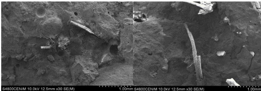
Figure 13: Fresh fracture micrograph corresponding to C-CBF (1%)
