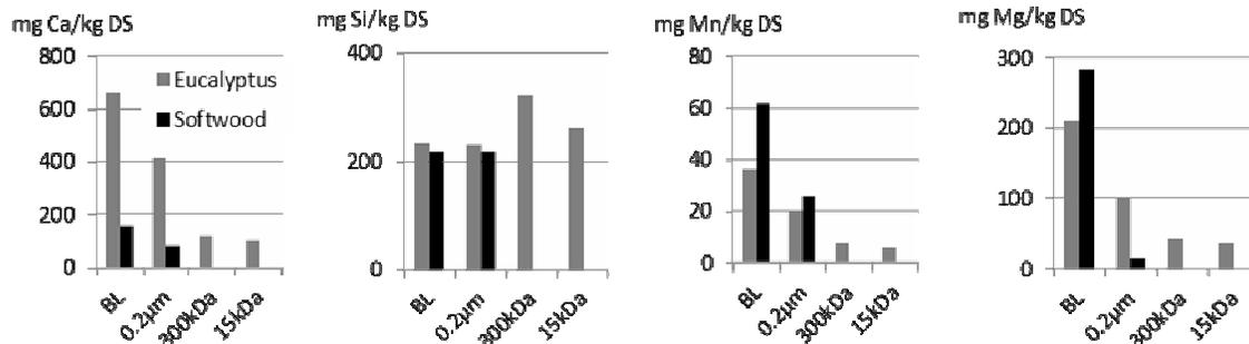
Figure 5: Ca, Si, Mn and Mg concentration in eucalyptus (grey) and softwood (black) black liquor and permeates. The DS in the permeates is lower than in black liquor
