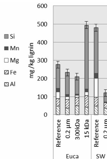
Figure 8: Concentration of Al, Fe, Mn, Mg and Si in the eucalyptus and softwood lignins separated from the black liquors (Reference) and permeates. Error bars represent the standard deviation for double samples precipitated at pH 10.2 and washed at pH 2.3
