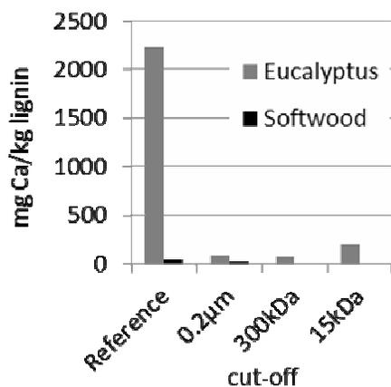
Figure 7: Ca concentration in the washed lignins separated from the untreated black liquors (Reference) and permeates. The samples were precipitated at a pH between 9.6 and 9.8 and washed at pH 2.3
