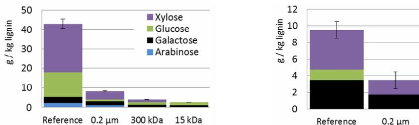
Figure 3: Carbohydrate content given as anhydrosugars in eucalyptus (left) and softwood lignin (right) separated from black liquors (Reference) and permeates. All samples were precipitated at a pH level between 9.6 and 9.8, and washed at pH 2.3
