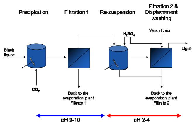
Figure 1: General principles of the LignoBoost process
