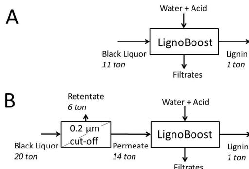
Figure 2: An example of a simplified mass balance for production of 1 ton of *Eucalyptus globulus* lignin using A) LignoBoost, yield 220 kg lignin/ton BLS, and B) Microfiltration (0.2 µm cut-off, VRF 0.7) followed by LignoBoost, yield 185 kg lignin/kg PS, permeate dry solids (PS) 37%
