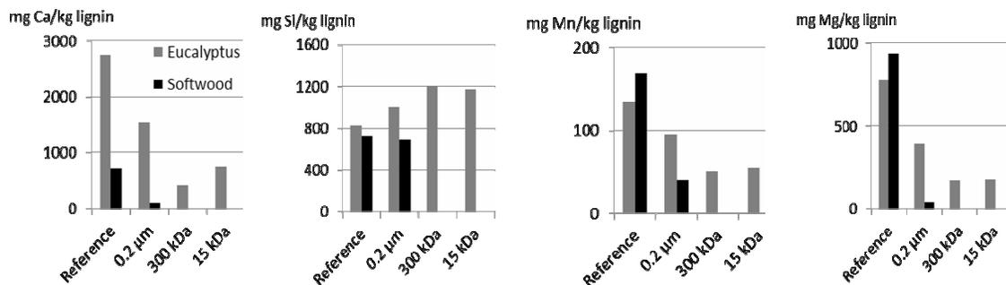
Figure 6: Ca, Si, Mn and Mg content in first stage filter cakes produced from the eucalyptus (grey) and softwood (black) black liquors (Reference) and permeates. All samples were precipitated at a pH between 9.6 and 9.8
