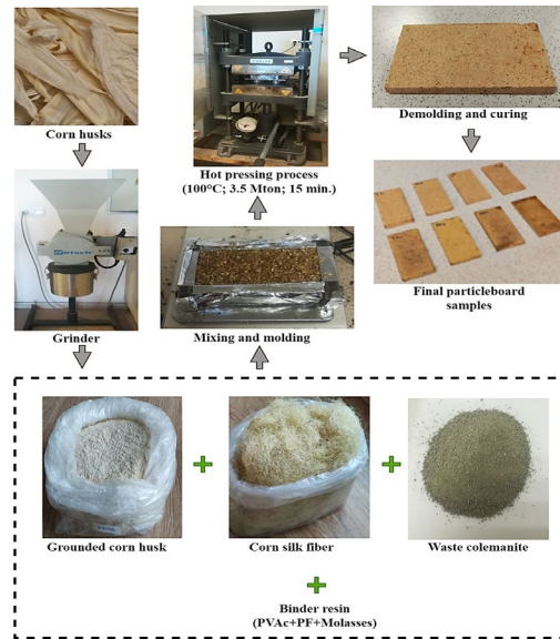
Figure 3: Manufacturing stages of corn husk-based eco-friendly PB samples
