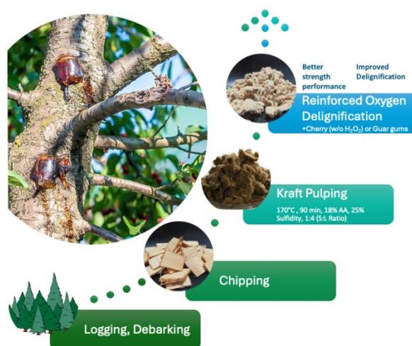
Figure 1: Procedure to produce pulp exhibiting high properties
