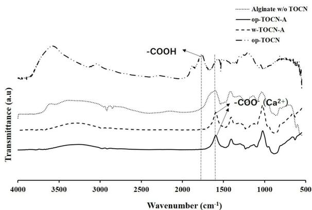
Figure 6: FTIR spectra of TOCN-alginate membranes and original TOCNs from OPEFB
