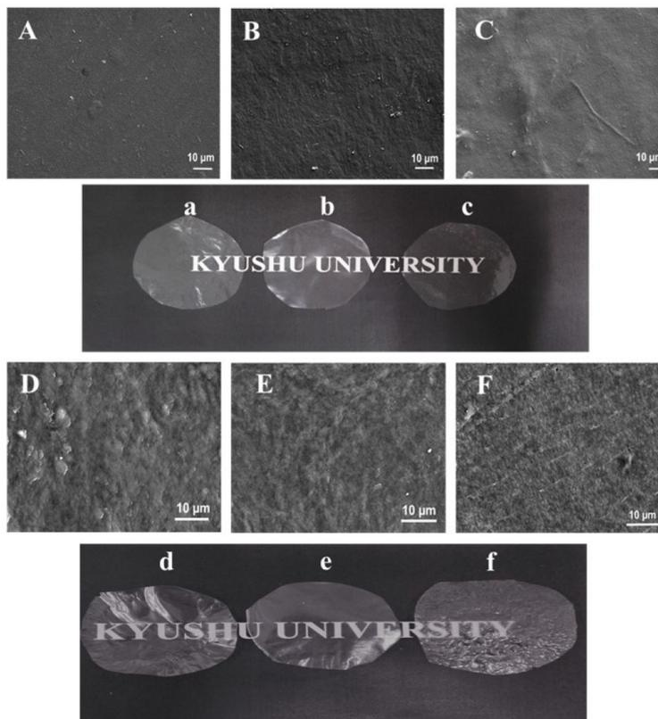
Figure 7: SEM images of membrane surfaces before (A: alginate w/o TOCN; B: op-TOCN-A; C: w-TOCN-A) and after the treatment (D: alginate w/o TOCN; E: op-TOCN-A; F: w-TOCN-A) and optical images of their representatives in lowercase letters (scale bars: 10  $\mu\text{m}$ )
