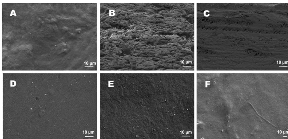
Figure 5: SEM images of cross-sectional (upper) and surface morphology (bottom) of (A, D) alginate w/o TOCN, (B, E) op-TOCN-A, and (C, F) w-TOCN-A (scale bars: 10 μm)
