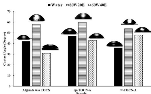
Figure 8: Contact angle measurement for water and water-ethanol mixtures
