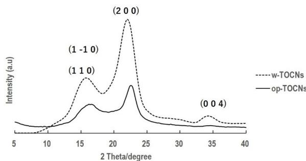
Figure 4: X-ray diffraction patterns of OPEFB-derived TOCNs (op-TOCNs) and wood-derived TOCNs (w-TOCNs)
