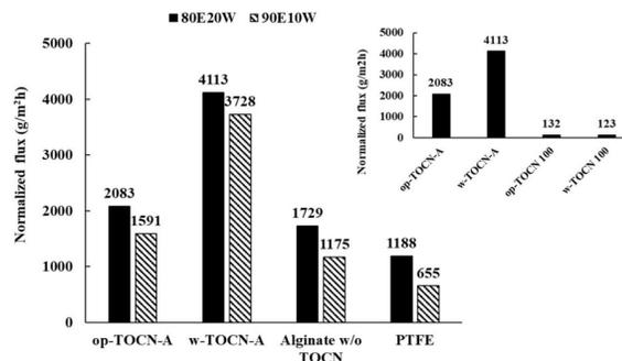
Figure 9: Normalized flux values of alginate, alginate-TOCN and PTFE membranes for water-ethanol mixtures
