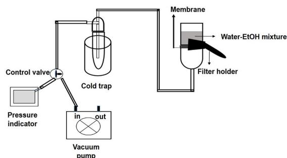
Figure 2: Membrane test scheme
