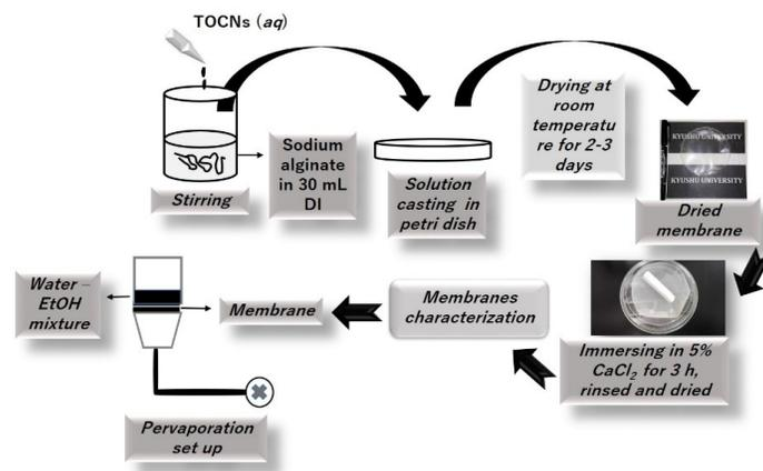
Figure 1: Experimental scheme of the preparation of alginate-TOCN membranes and their use for water-ethanol separation
