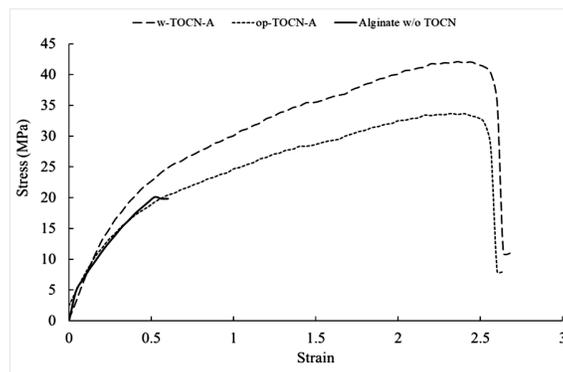
Figure 10: Tensile strength of alginate and alginate-TOCN membranes
