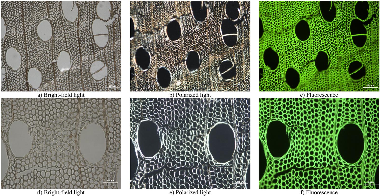
Figure 4: Microstructures in transverse sections of maple wood under bright-field light, polarized light and fluorescence (a), (b), (c): sample No. 2; (d), (e), (f): model specimen
