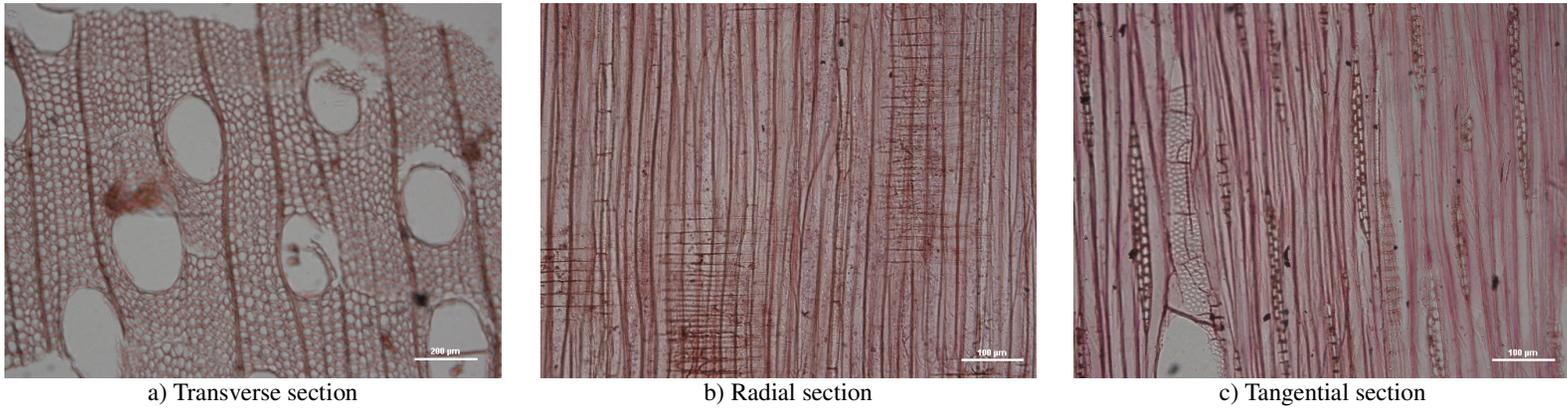
Figure 2: Microstructures of sample No.2 under bright-field light
