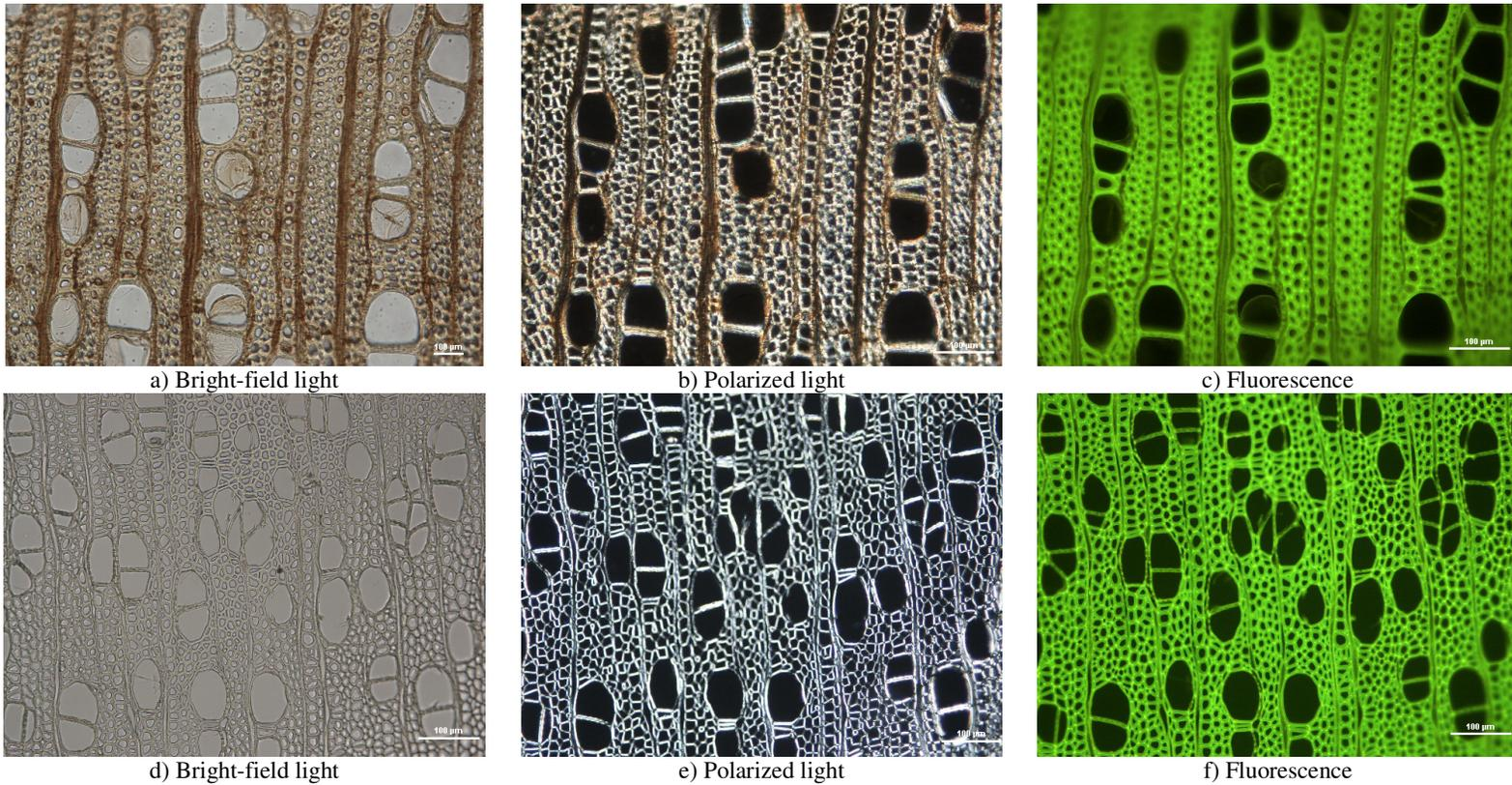
Figure 3: Microstructures in transverse sections of birch wood under bright-field light, polarized light and fluorescence (a), (b), (c): sample No. 1; (d), (e), (f): model specimen
