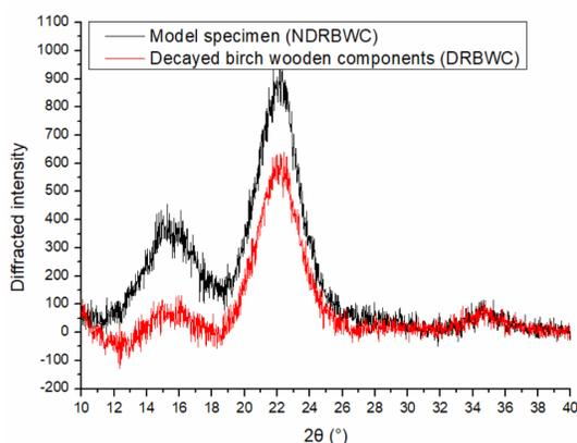
Figure 5: X-ray diffraction patterns of red birch wood
