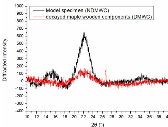
Figure 6: X-ray diffraction patterns of maple wood
