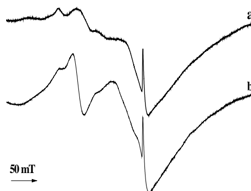
Figure 6: EPR spectra of RP (a) and PA (b) samples after silver adsorption
