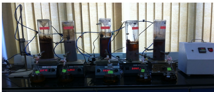
Figure 2: Semi-continuous reactor study setup with controlled aeration and agitation
