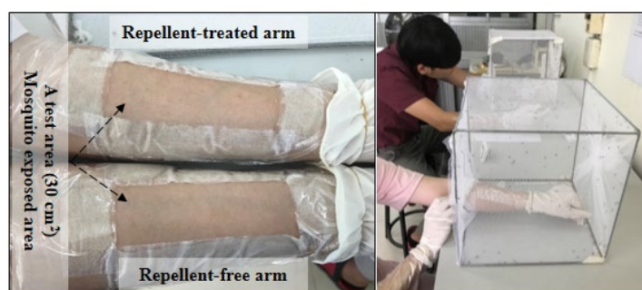
Figure 1: Test of mosquito repellency with Ae. aegypti by “arm-in-cage” technique according to the WHO standard test method
