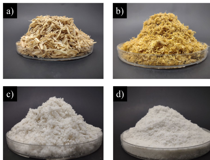
Figure 2: Images of (a) raw, and (b) alkali-treated rice husk; and cellulose after (c) the first wash and (d) the second wash
