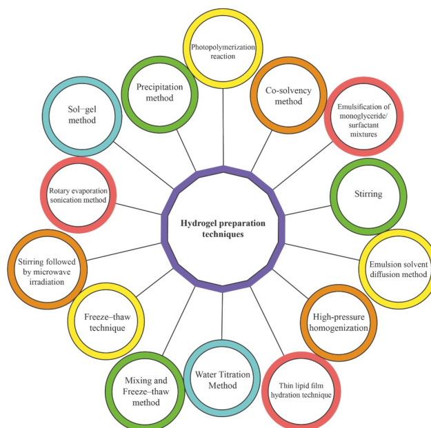
Figure 2: Techniques for the preparation of hydrogels
