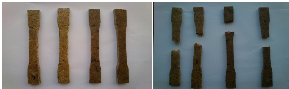
Figure 3: Tensile test specimens before and after testing
