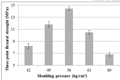
Figure 3: Relation between moulding pressure and flexural strength of composite specimens (production conditions: binder amount: 80 g, f/b: 0.50, moulding pressure temperature: 100 °C, moulding pressure time: 20 min,  $\bar{d}$ : 525  $\mu\text{m}$ )
