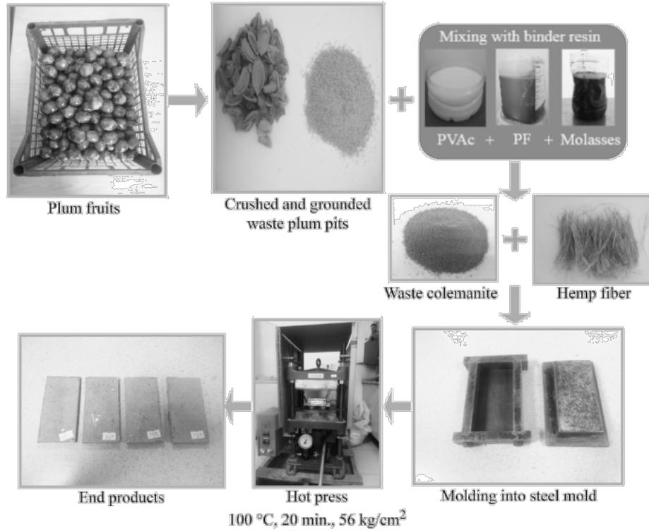
Figure 1: Composite specimen production process
