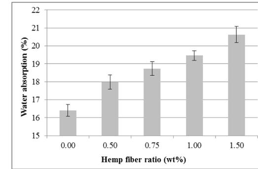
Figure 6: Relation between hemp fiber ratio and WA value of composite specimens (production conditions: binder amount: 80 g, f/b: 0.50, moulding pressure temperature: 100 °C, moulding pressure time: 20 min, moulding pressure: 56 kg/cm<sup>2</sup>, d: 525 µm)
