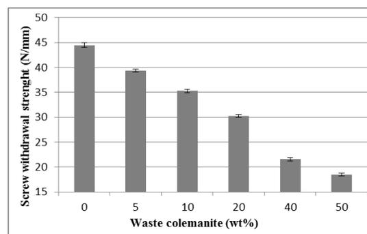
Figure 10: Screw withdrawal strength as a function of colemanite ratio (production conditions: binder: 80 g, f/b: 0.50, moulding pressure: 56 kg/cm<sup>2</sup> at 100 °C for 20 min, d: 525 μm, hemp fiber: 0.75%)
