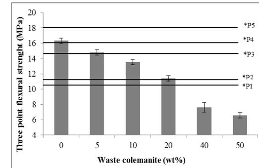
Figure 8: Flexural strength as a function of colemanite ratio (production conditions: binder: 80 g, f/b: 0.50, moulding pressure: 56 kg/cm<sup>2</sup> at 100 °C for 20 min, d: 525 µm, hemp fiber: 0.75%); EN312 flexural strength limit values: \*P1 $\geq$ 10.5 MPa (general use), \*P2 $\geq$ 11 MPa (interior use), \*P3 $\geq$ 15 MPa (wet-non load bearing), \*P4 $\geq$ 16 MPa (dry-load bearing), \*P5 $\geq$ 18 MPa (wet-load bearing)
