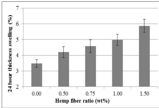
Figure 5: Relation between hemp fiber ratio and TS value of composite specimens (production conditions: binder amount: 80 g, f/b: 0.50, moulding pressure temperature: 100 °C, moulding pressure time: 20 min, moulding pressure: 56 kg/cm<sup>2</sup>, d: 525 µm)
