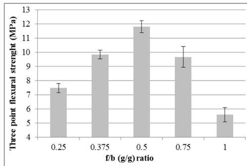
Figure 2: Relation between f/b ratio and flexural strength of composite specimens (starting production conditions: moulding pressure temperature: 100 °C, moulding pressure time: 20 min, and pressure: 49 kg/cm<sup>2</sup>, binder amount: 80 g, d: 525  $\mu\text{m}$ )
