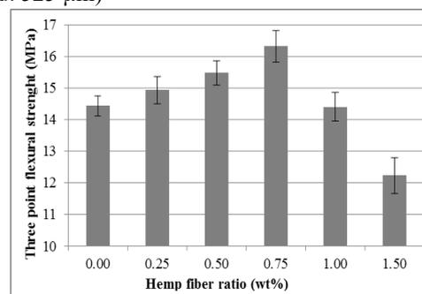
Figure 4: Relation between hemp fiber ratio and flexural strength of composite specimens (production conditions: binder amount: 80 g, f/b: 0.50, moulding pressure temperature: 100 °C, moulding pressure time: 20 min, moulding pressure: 56 kg/cm<sup>2</sup>,  $\bar{d}$ : 525  $\mu\text{m}$ )
