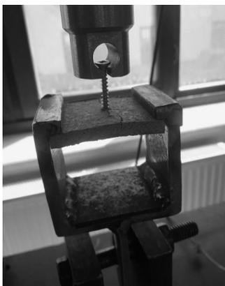
Figure 9: Screw withdrawal experiment
