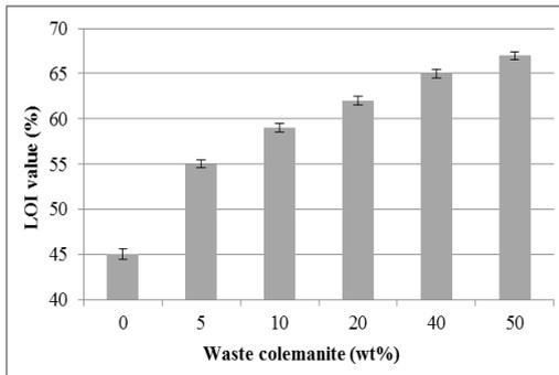
Figure 7: Relation between waste colemanite ratio and LOI value of composite specimens (production conditions: binder amount: 80 g, f/b: 0.50, moulding pressure temperature: 100 °C, moulding pressure time: 20 min, moulding pressure: 56 kg/cm<sup>2</sup>, d: 525 µm, hemp fiber: 0.75%)
