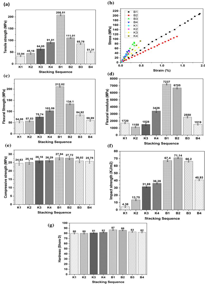
Figure 3: (a) Tensile strength, (b) Stress-strain curves, (c) Flexural strength, (d) Flexural modulus, (e) Compressive strength, (f) Impact strength, and (g) Hardness comparison chart of composites
