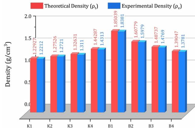
Figure 2: Theoretical densities and experimental densities of laminates
