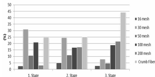
Figure 3: Evolution of fiber size during the recycling stages
