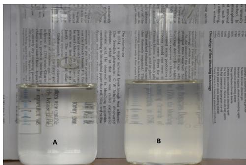
Figure 4: Appearance of cellulose nanofibril suspensions; (A) 0.1 wt%; (B) 0.2 wt%
