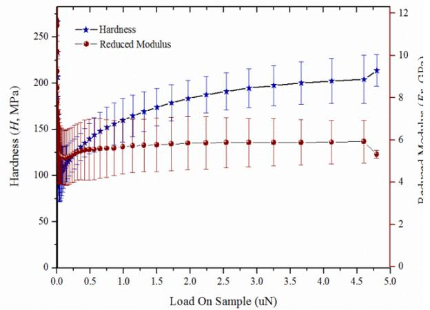
Figure 4: Hardness and reduced modulus versus indented load
