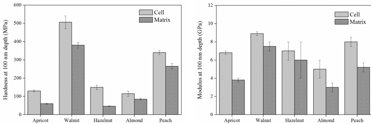
Figure 7: Summary of the resulted hardness and modulus for the specimens under study
