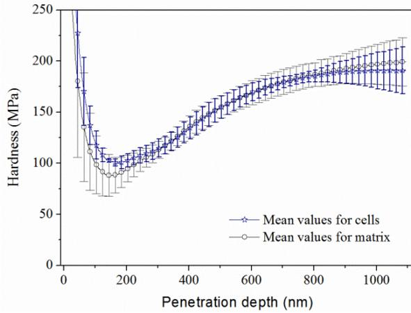
Figure 3: Hardness mean values for cell and matrix microstructures of the apricot shell
