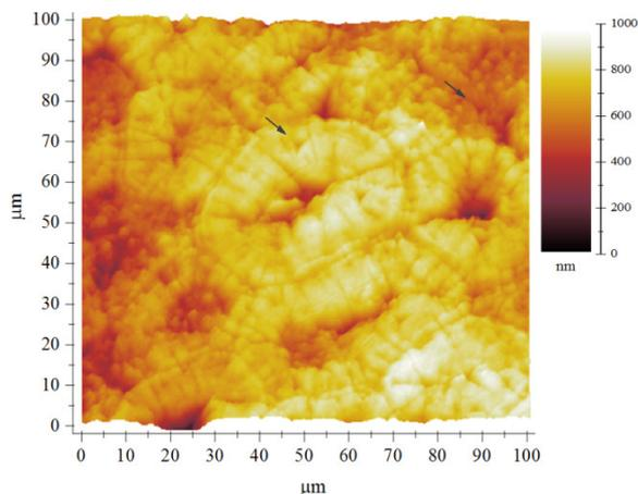
Figure 1: 3D image of the microstructure acquired on apricot shell. The arrows indicate several imprints on cells and matrix generated by nanoindentation at 1000 nm depth
