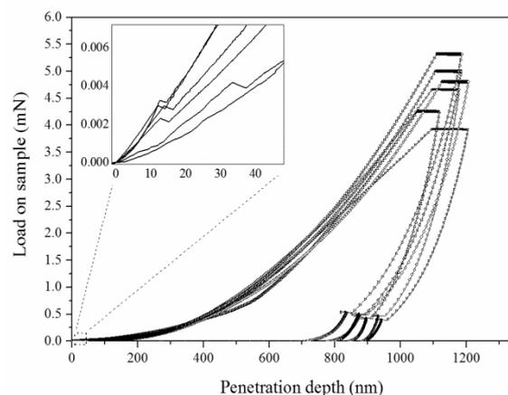
Figure 2:  $P-h$  nanoindentation curves recorded the apricot shell indented on cross-section. The in-set figure is a detail of the pop-in events recorded
