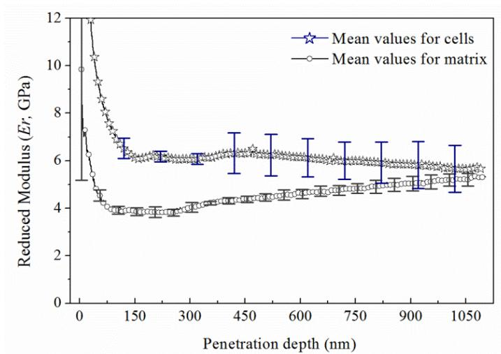
Figure 5: Modulus mean values for cell and matrix microstructures of the apricot shell
