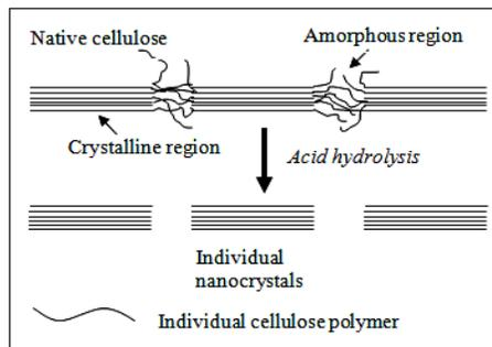
Figure 4: Schematic diagram of acid hydrolysis of cellulose and generation of nanocrystals<sup>50</sup>
