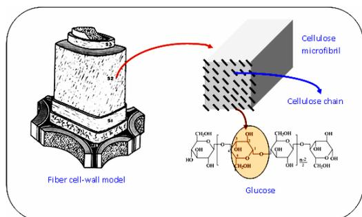
Figure 3: The structure of wood cell and cellulose microfibril<sup>8,11</sup>
