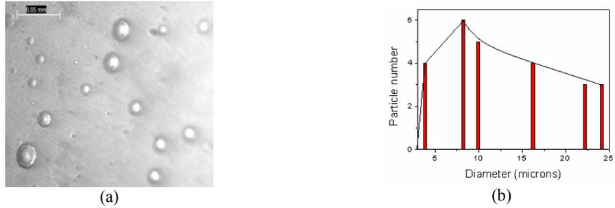
Figure 1: Microscopic image (a) and distribution curve (b) of the dispersed phase of PVA/CS 50/50 blend
