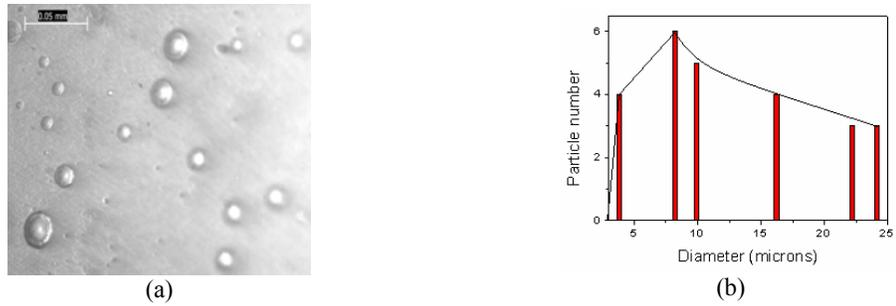
Figure 1: Microscopic image (a) and distribution curve (b) of the dispersed phase of PVA/CS 50/50 blend
