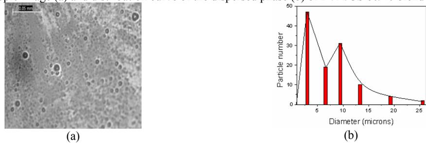
Figure 3: Microscopic image (a) and distribution curve of the dispersed phase (b) of PVA/CS 70/30 blend
