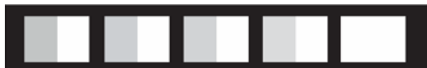
Figure 21: Grey scale analysis, which determines the color change compared with fabric before testing (from the left (highest color difference) – to the right (no color difference))
