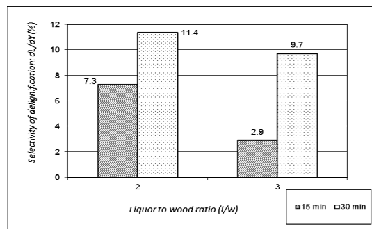
Figure 6: Effect of liquor to wood ratio (l/w) on delignification selectivity (10% miscanthus and 90% birch wood; initial impregnation, 31% Na 2 SO 3 on o.d. mass)
