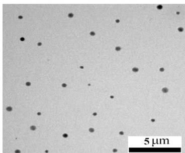
Figure 1: TEM image of PU-Hep nanoparticles
