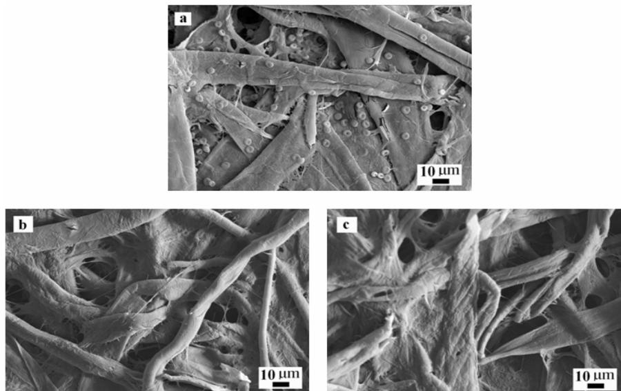
Figure 7: SEM images of the samples after incubation with rabbit whole blood for 30 min; (a) Crude filter paper, (b) Paper-Hep, (c) Paper-PU-Hep
