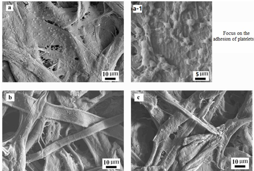
Figure 6: SEM images of the samples after incubation with PRP for 90 min; (a) Crude filter paper, (b) Paper-Hep, (c) Paper-PU-Hep
