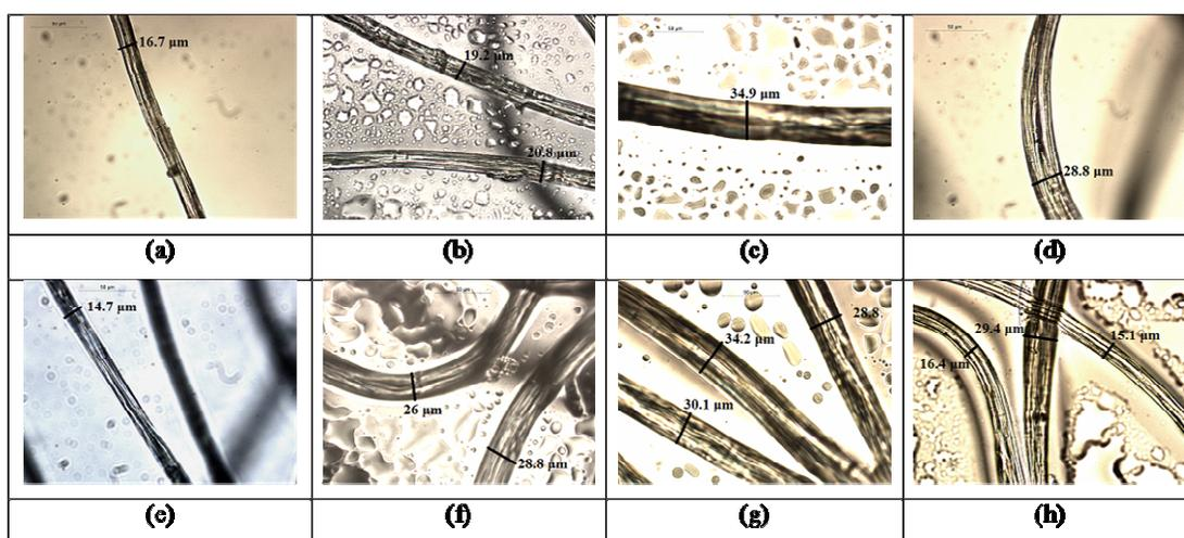
Figure 6: Optical microscopy images of the cellulose/chitin mix fibers treated with NIPAAm – (a) dry and swollen at different temperatures (b) 30 °C, (c) 32 °C, (d) 36 °C; and with PNIPAAm – (e) dry and swollen at different temperatures (f) 30 °C, (g) 32 °C, (h) 36 °C
