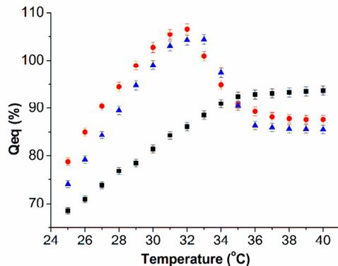
Figure 1: Equilibrium swelling degree versus temperature in double distilled water (pH ~5.5) for unmodified CC (■), NIPAAm-modified fibers (●) and PNIPAAm-modified fibers (▲)
