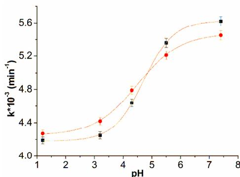
Figure 5: Swelling rate constant ( $k$ ) vs pH for the swelling of CC/NIPAAm (■) and CC/PNIPAAm (●)
