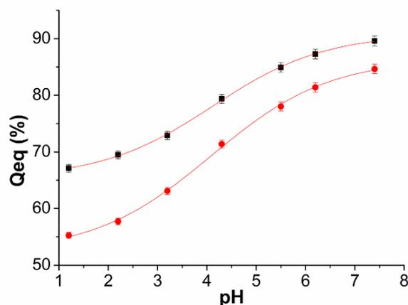
Figure 2: Maximum swelling degree versus pH of solutions, at room temperature (25 °C) for NIPAAm grafted samples (■) and PNIPAAm grafted samples (●)
