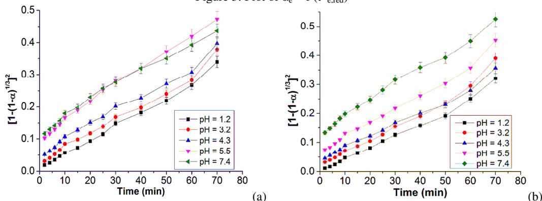
Figure 4: Plot of  $[1-(1-\alpha)^{1/3}]^2$  as a function of time for swelling of (a) CC/NIPAAm and (b) CC/PNIPAAm fibers in different pH solutions at 25 °C
