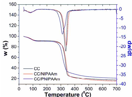
Figure 7: TG/DTG curves for untreated and modified cellulose/chitin mix fibers
