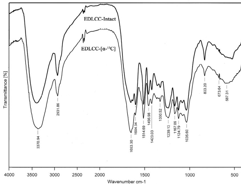
Figure 4: FT-IR spectra of EDLCC-IS from rice stalk
