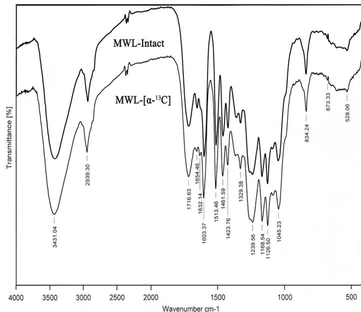
Figure 2: FT-IR spectra of MWL from rice stalk
