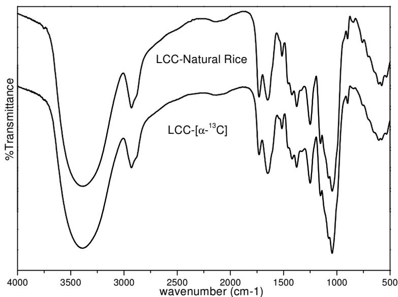
Figure 3: FT-IR spectra of LCCs from rice stalk
