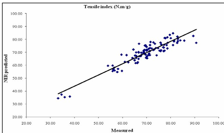
Figure 3: Calibration model for tensile index of unbleached beech kraft pulps (R = 0.9226)
