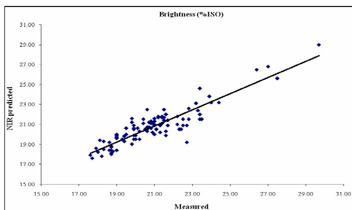
Figure 6: Calibration model for brightness of unbleached beech kraft pulps ( $R = 0.9377$ )
