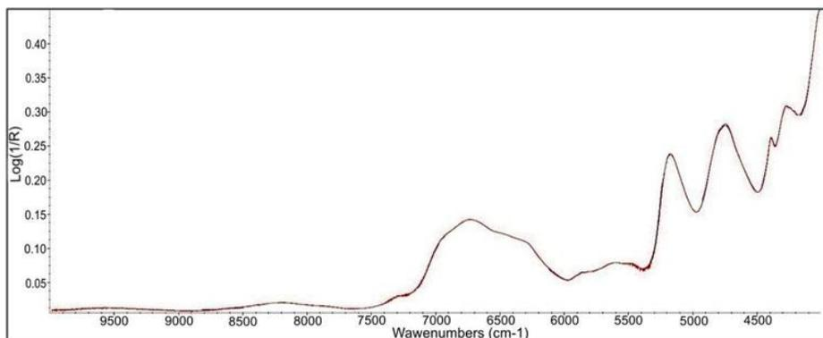
Figure 1: Average spectrum of unbleached beech kraft pulp
