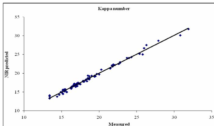
Figure 2: Calibration model for kappa number of unbleached beech kraft pulps (R = 0.9957)
