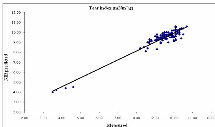
Figure 5: Calibration model for tear index of unbleached beech kraft pulps ( $R = 0.9515$ )
