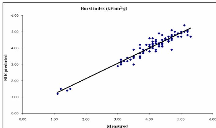
Figure 4: Calibration model for burst index of unbleached beech kraft pulps ( $R = 0.9580$ )
