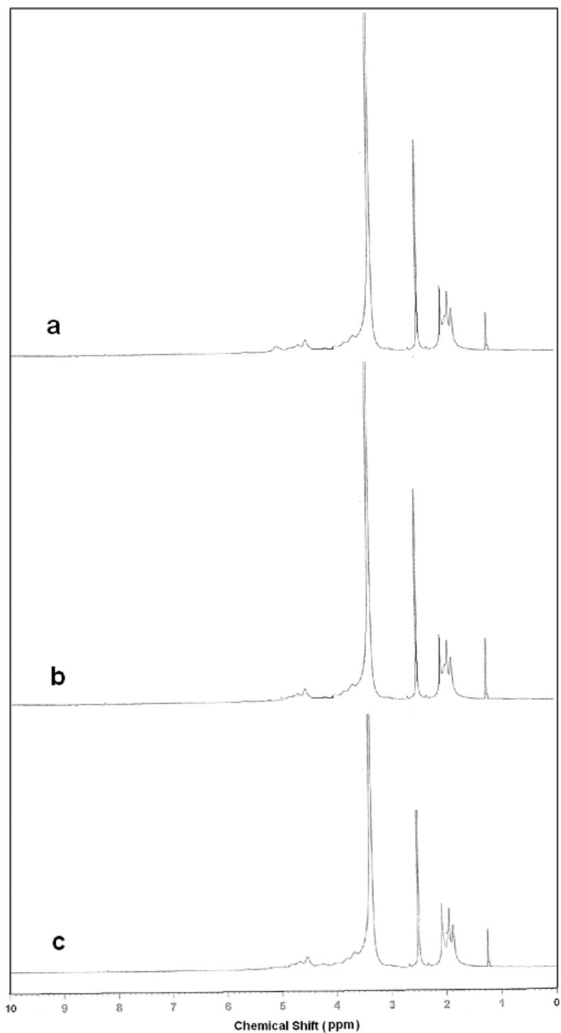
Figure 2: <sup>1</sup>H-NMR spectra of (a) PMMA grafted CA in DMSO in presence of CAN (CA-g-PMMA-273); (b) PMMA grafted CA in DMAc in presence of BPO (CA-g-PMMA-85); (c) PMMA grafted CA in acetone in presence of Sn(Oct)<sub>2</sub> (CA-g-PMMA-250)
