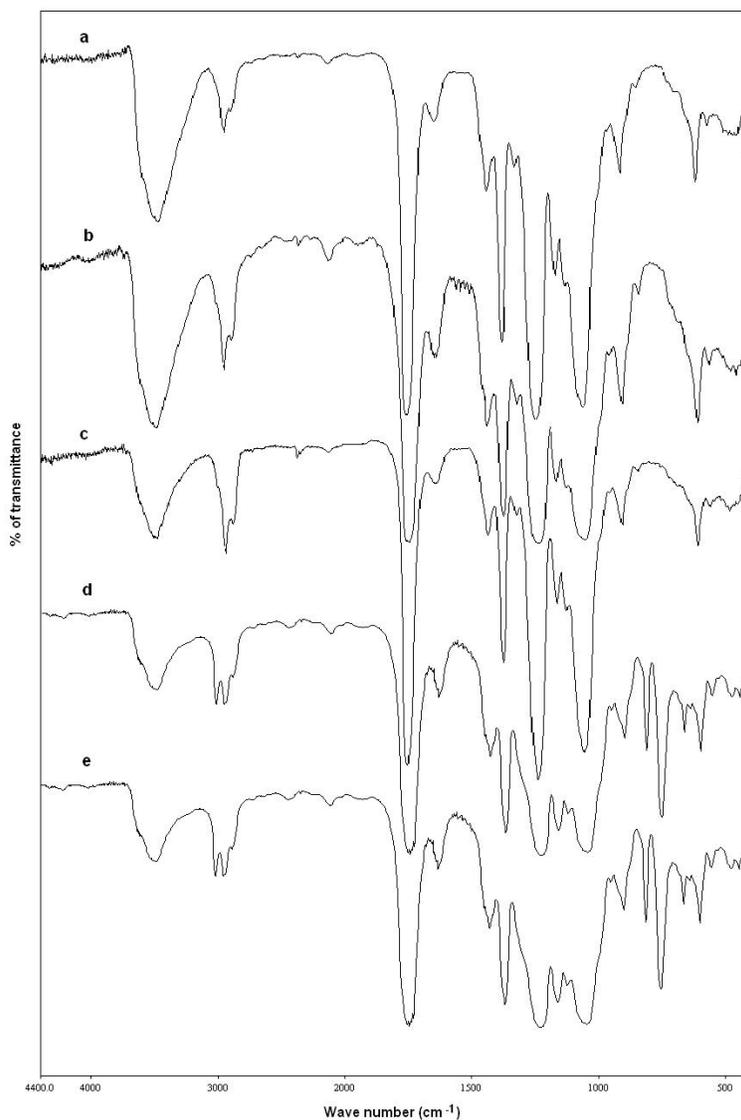
Figure 1: FTIR spectra of (a) CA; (b) PMMA grafted CA in DMSO in presence of CAN (CA-g-PMMA-273); (c) PMMA grafted CA in DMAc in presence of BPO (CA-g-PMMA-85); (d) PMMA grafted CA in 1,4-dioxane in presence of BPO (CA-g-PMMA-110); (e) PMMA grafted CA in acetone in presence of  $\text{Sn}(\text{Oct})_2$  (CA-g-PMMA-250)
