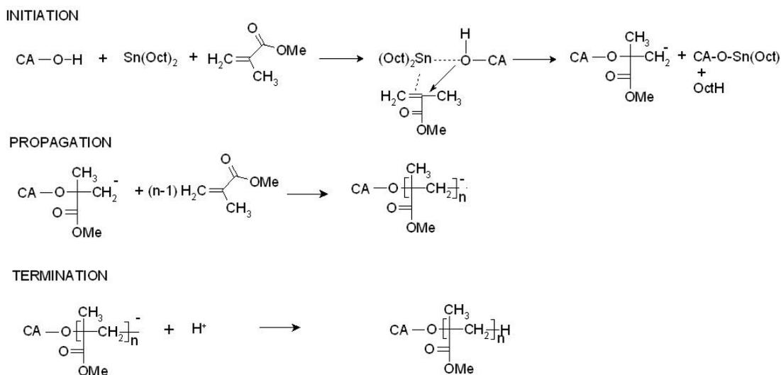
Scheme 3: Mechanism of grafting of PMMA onto CA by Sn(Oct)<sub>2</sub> as initiator
