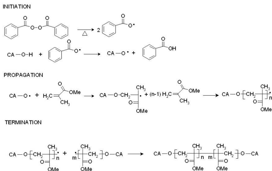
Scheme 2: Mechanism of grafting of PMMA onto CA by BPO as initiator
