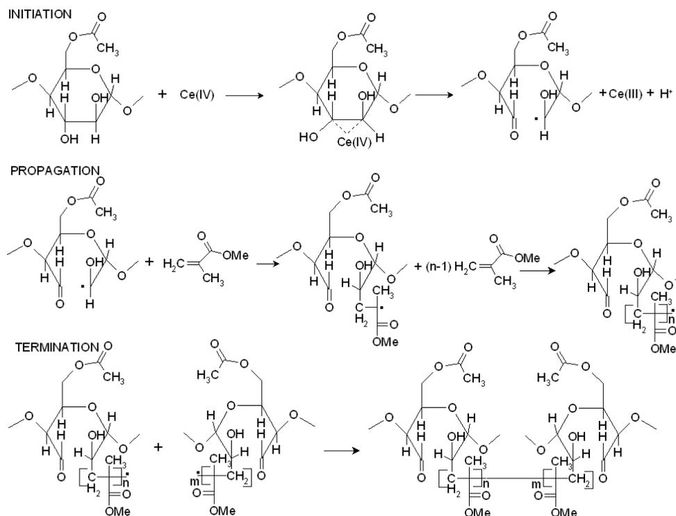
Scheme 1: Mechanism of grafting of PMMA onto CA by Ce<sup>+4</sup> ion
