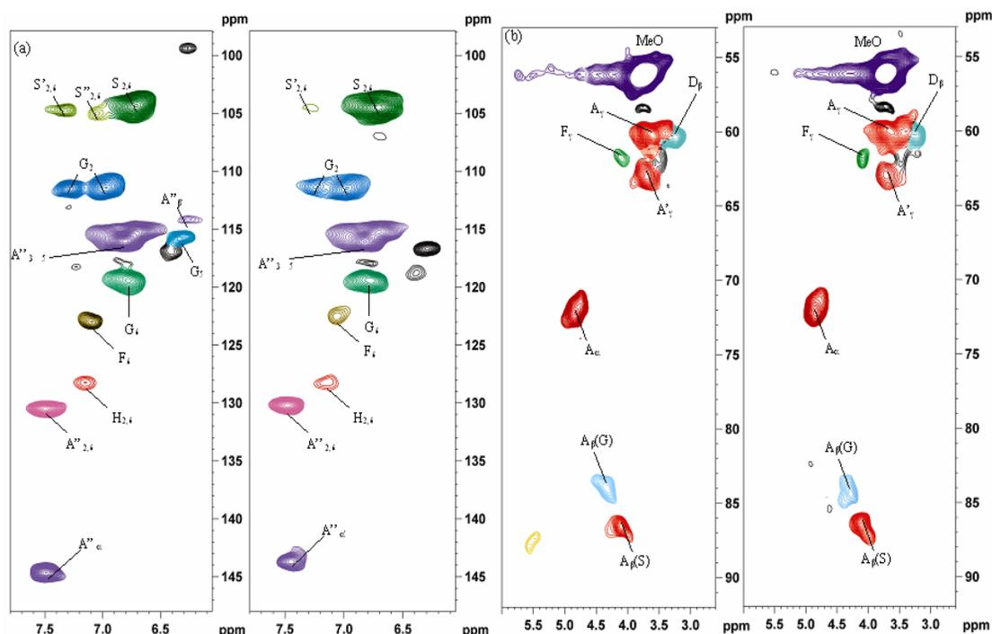
Figure 8: HSQC NMR spectra of lignin fractions L2 (left) and L3 (right) isolated with 0.25% NaOH-EtOH (95%) and 0.5% NaOH at 80 °C for 3 h from *Carex meyeriana* Kunth: (a) oxygenated aliphatic region  $\delta_C/\delta_H$  53-92/2.6-6 ppm (b) aromatic region  $\delta_C/\delta_H$  98-148/6-7.8 ppm
