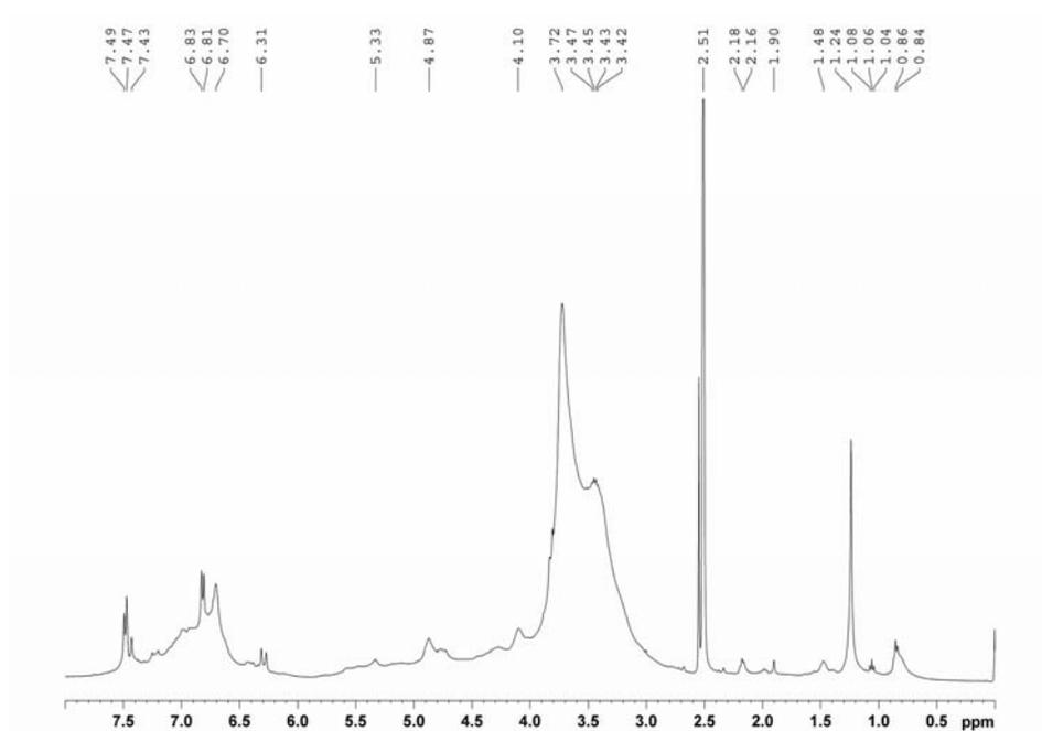
Figure 5:  $^1\text{H}$  NMR spectrum of lignin fraction L3 isolated with 0.5% NaOH at 80 °C for 3 h
