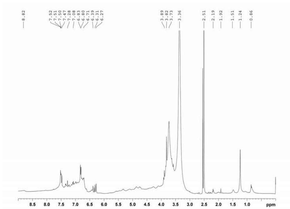
Figure 4:  $^1\text{H}$  NMR spectrum of lignin fraction L2 isolated with 0.25% NaOH-EtOH (95%) at 80 °C for 3 h
