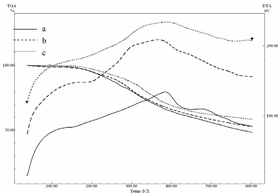
Figure 10: TGA/DTA curves of lignin fractions L2 (a), L3 (b) and L5 (c) isolated with 0.25% NaOH-EtOH (95%), 0.5% NaOH and 1.5% NaOH at 80 °C for 3 h, respectively
