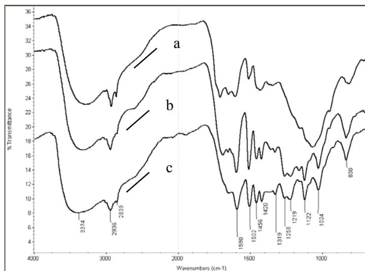
Figure 2: FT-IR spectra of *Carex meyeriana* Kunth lignin fractions isolated with distilled water (a), 0.25% NaOH-EtOH (95%) (b) and 0.5% NaOH (c) at 80 °C for 3 h
