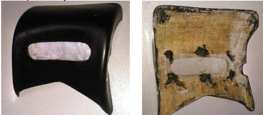
Figure 11: NFRVM polyester composite products: engine guard of two-wheelers
