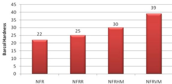
Figure 8: Barcol hardness for different forms of composites
