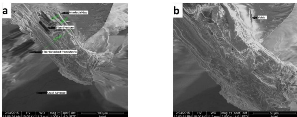
Figure 5: SEM images of flexure-tested specimens of Nendran fiber mat composites
