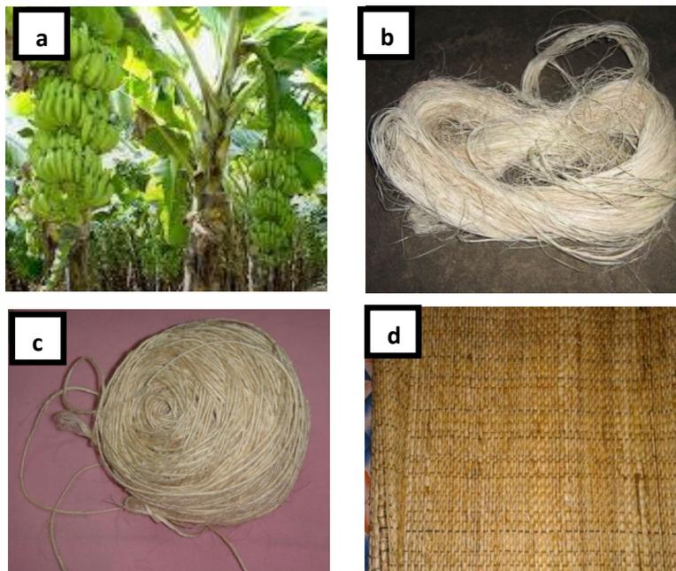
Figure 1: Preparation of Nendran fiber rope mat; (a) Nendran banana tree, (b) extracted fiber, (c) prepared fiber rope, and (d) woven fiber rope mat
