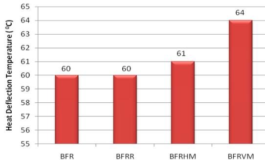
Figure 10: Heat deflection temperature test (HDT) for different forms of composites
