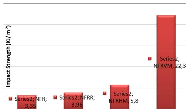
Figure 6: Impact strength for different fiber reinforced composites
