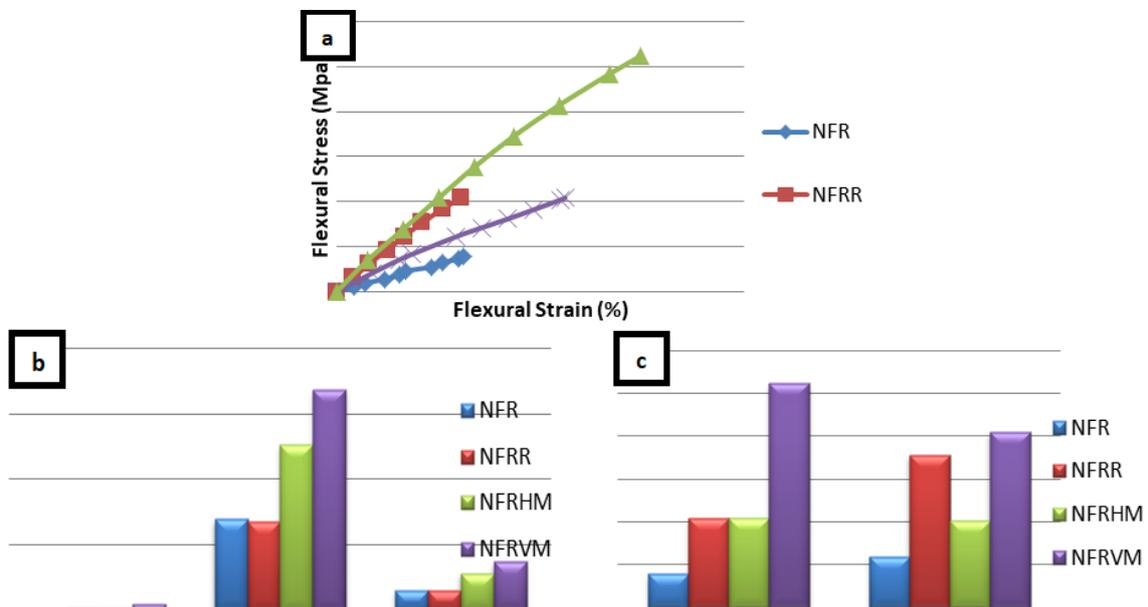
Figure 4: Flexural properties: (a) stress vs strain curves, (b) break load, maximum displacement and percentage elongation at break, (c) flexural strength and flexural modulus of the four different composites
