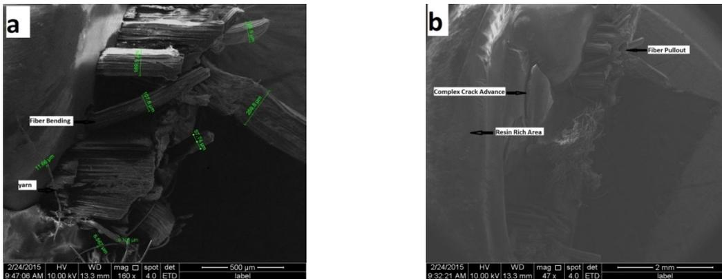
Figure 3: SEM images of tensile-tested specimens of Nendran fiber mat composites
