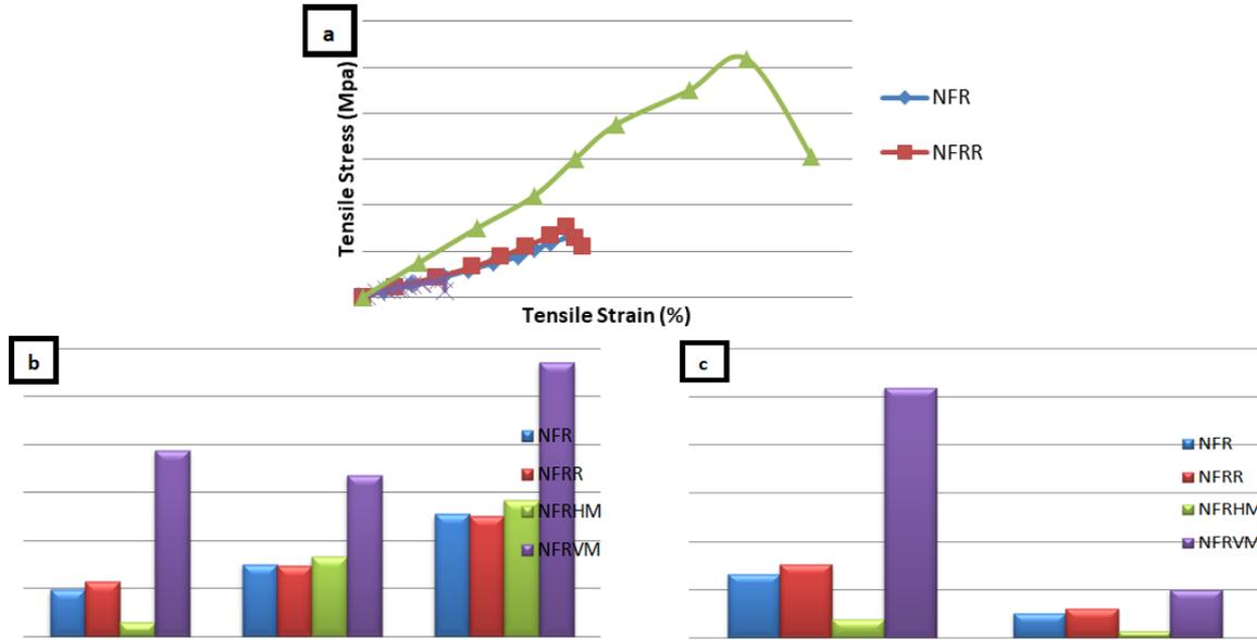
Figure 2: Tensile properties: (a) stress vs strain curves, (b) break load, maximum displacement and percentage elongation at break, (c) tensile strength and tensile modulus of the four different composites
