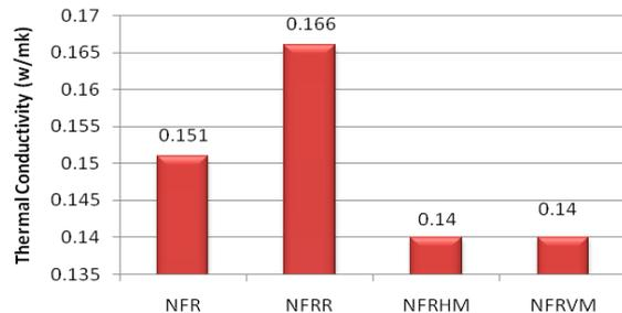
Figure 9: Thermal conductivity for different forms of composites
