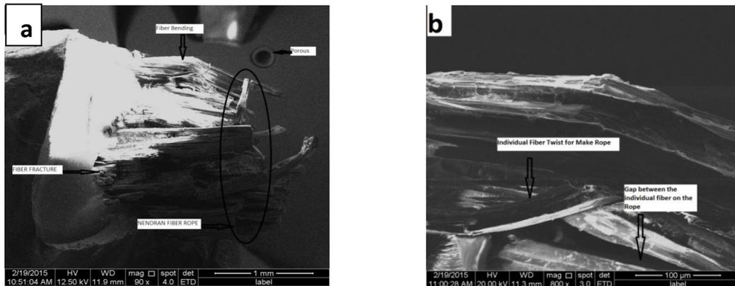
Figure 7: SEM images of impact-tested specimens of Nendran fiber mat composites
