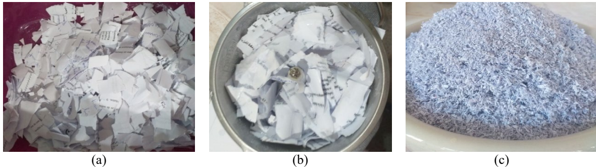
Figure 2: Steps of paper preparation – (a) cut paper, (b) paper with water in a mixer machine, and (c) minced paper
