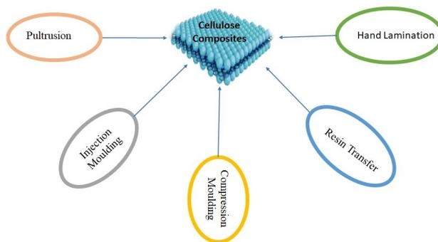
Figure 1: Methods of fabrication of cellulose composite materials
