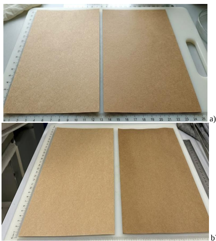
Figure 5: Photographs of (a) uncoated and coated heat-resistant paper, (b) coated paper before and after heat exposure
