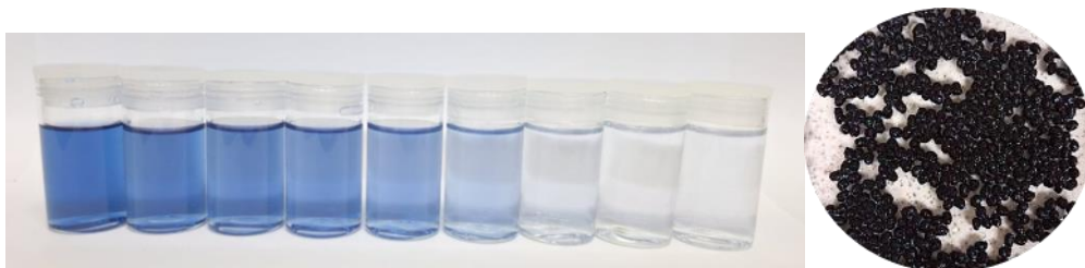
Figure 7: RB5 solutions at different contact times, and KH-CH-ECH composite beads after adsorption
