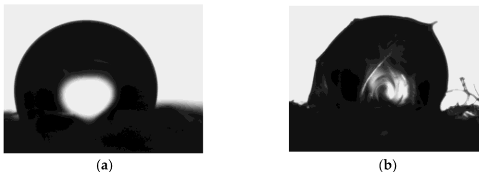
Figure 2: Visuals depicting contact angle measurements of (a) soap-washed wool fibers and (b) wool fibers exposed to peroxide treatment (adopted from ref. 49 with permission; Copyright 2022 MDPI Materials (Open Access Creative Commons CC-BY-NC 4.0 license)) 49
