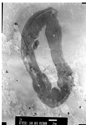
Figure 12: Transverse section of straw fiber after one recycling (TEM, size of image: 2 \times 2 \mu\text{m} )
