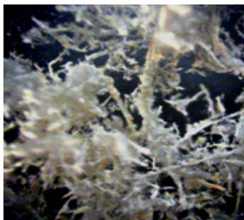
Figure 1: Optical image of the birch sanding dust (x40 magnification)
