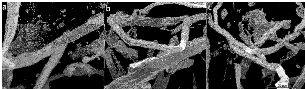
Figure 1: SEM photographs of straw cellulose before deashing (a), and after deashing with NaF-HCl aqueous solution (b) and HF-HCl aqueous solution (c)
