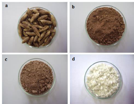
Figure 2: Photographs of a) untreated DS, b) ground DS, c) alkali treated DS, d) cellulose DS
