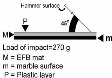
Figure 1: Illustration of the mechanical impact named staccato hammering impact due to the elasticity or short-time contact between the hammer impact surface and the EFB mat
