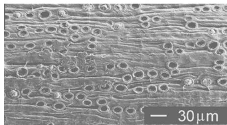
Figure 4: EFB surface after treatment with DTPA
