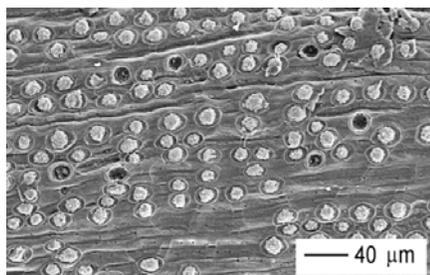
Figure 3: Initial surface of the intact EFB vascular bundle
