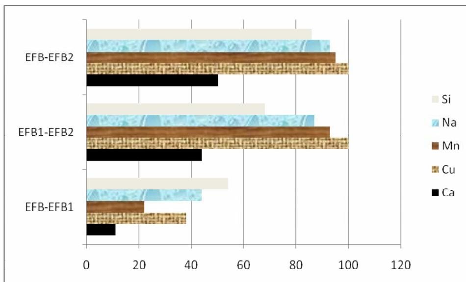
Figure 2: Percentage reduction of elements after the treatment
