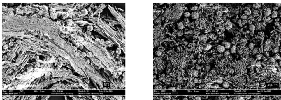
Figure 7: Ash of EFB without treatment (left) and after chelation with DTPA (right)
