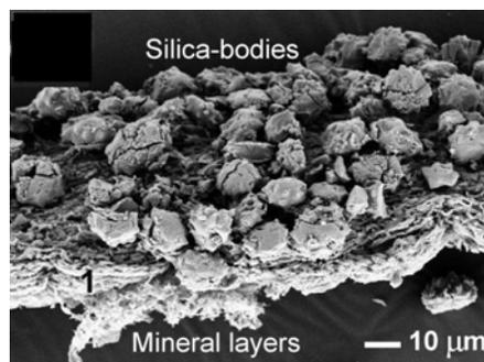
Figure 6: Micrograph of intact ash showing silica lying on the top of the mineral layer
