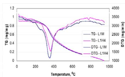
Figure 3: Thermograms recorded for non-modified lignin L<sub>1</sub> and for hydroxymethylated derivative L<sub>1</sub>H<sub>4</sub>
