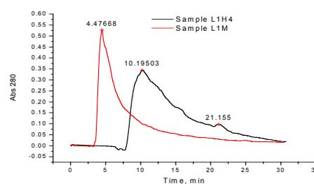
Figure 4: Chromatogram of unmodified L<sub>1</sub> (1) and modified L<sub>1</sub>H<sub>4</sub> (2) lignin obtained by HPLC
