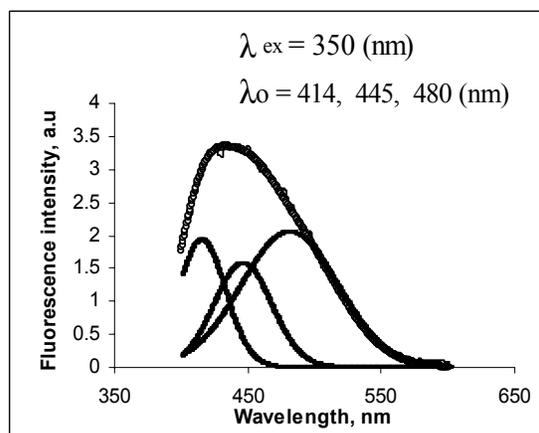
Figure 6: Fluorescence spectra for wheat straw lignin ( $L_1$ )
