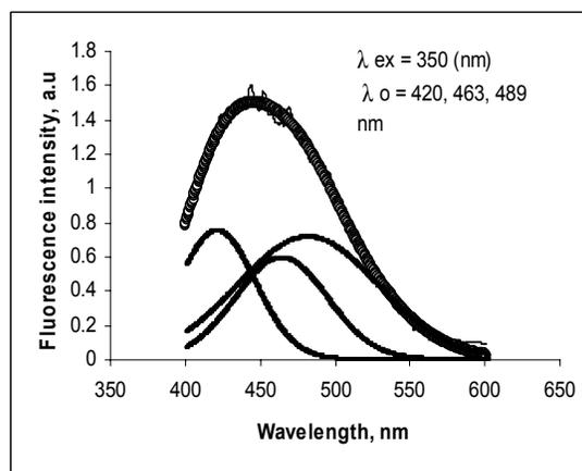
Figure 7: Fluorescence spectra for hydroxymetylated wheat straw lignin ( $L_1H_4$ )
