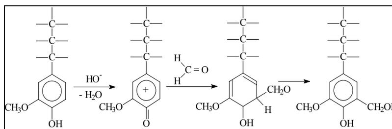
Figure 1: General scheme of the chemical modification of lignin through hydroxymethylation
