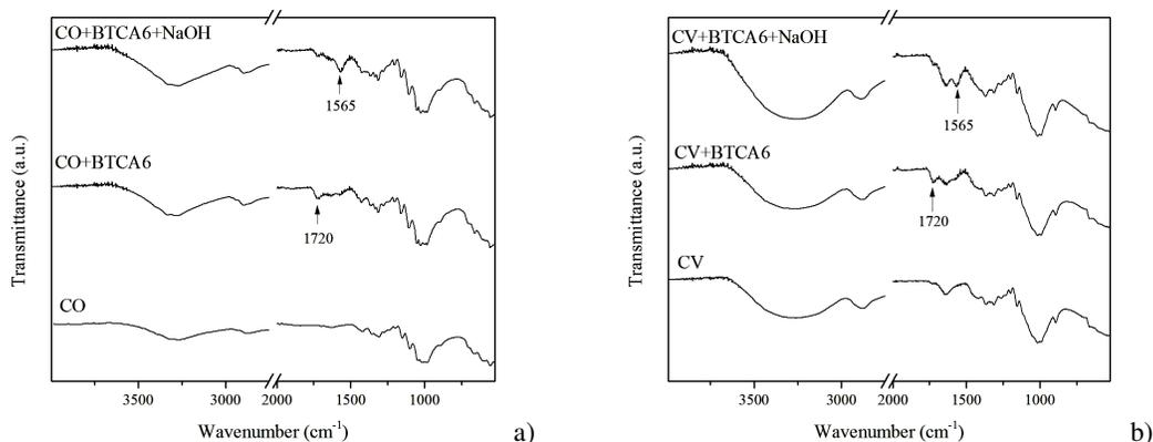
Figure 1: FTIR spectra of (a) control CO sample, CO+BTCA6+Cu sample and Co+BTCA6+Cu sample immersed into 0.1 N NaOH solution; and (b) control CV sample, CV+BTCA6+Cu sample and CV+BTCA6+Cu sample immersed into 0.1 N NaOH solution
