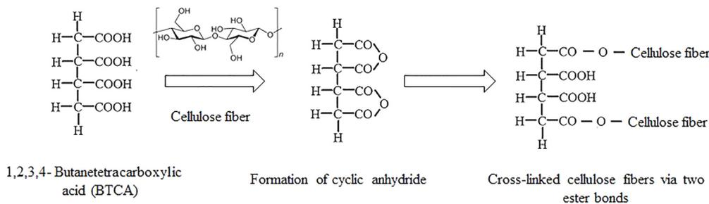
Figure 2: The schematic illustration of esterification of cellulose fibers with BTCA
