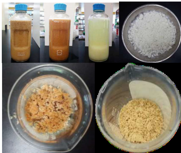
Figure 1: Bleaching process (top left) to extract cellulose (top right) from sugarcane bagasse, and dried carboxymethyl cellulose (CMC) from sugarcane bagasse (bottom left) and palm kernel cake (bottom right)
