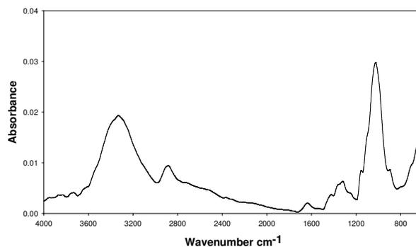
Figure 4: FTIR spectrum of untreated, pristine cellulose powder
