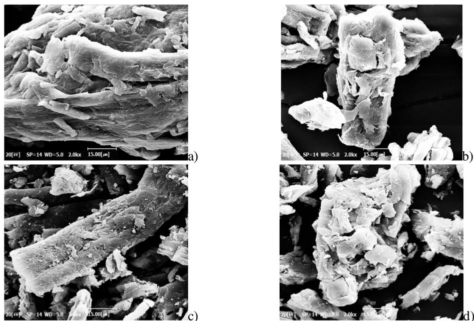
Figure 9: SEM micrographs of esterified cellulose with 2 moles of phthalic anhydride under OAC at various microwave irradiation times; (a) pristine, (b) 30 seconds, (c) 60 seconds and (d) 120 seconds
