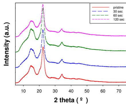
Figure 8: XRD of esterified cellulose with 2 moles of phthalic anhydride under OAC medium at various microwave irradiation times
