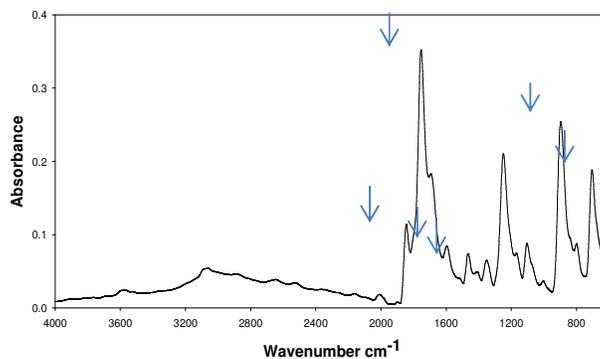
Figure 3: FTIR spectrum of phthalic anhydride
