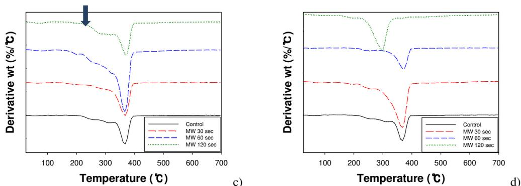
Figure 10: TGA and 1<sup>st</sup> derivative curves of cellulose treated by phthalic anhydride under OAC medium at various microwave irradiation times: (a) and (c) 1 mole of phthalic anhydride, (b) and (d) 2 moles of phthalic anhydride
