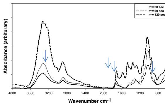
Figure 5: FTIR spectra of esterified cellulose by phthalic anhydride (1 mole) under OAC medium at various microwave irradiation times
