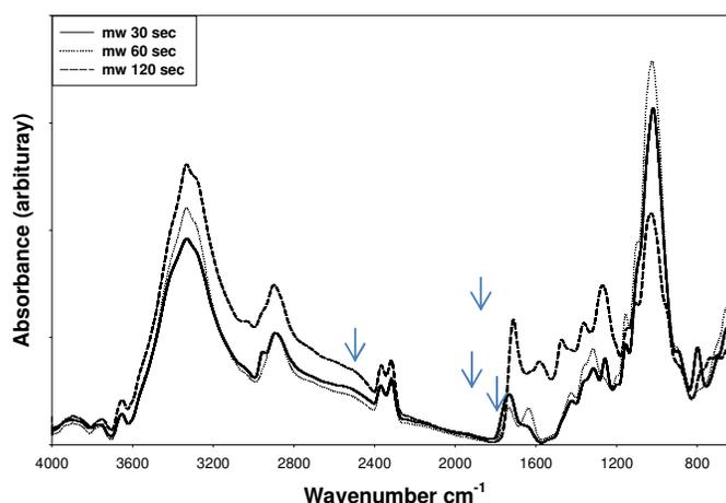
Figure 7: FTIR spectra of esterified cellulose by 2 moles of phthalic anhydride under OAC medium for various microwave irradiation times
