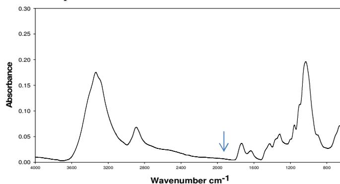
Figure 6: FTIR spectrum of cellulose treated by OAC for 60 seconds of microwave irradiation time (no phthalic anhydride)
