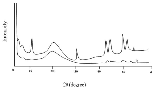
Figure 6: XRD spectra of (a) fibrous assembly and (b) film
