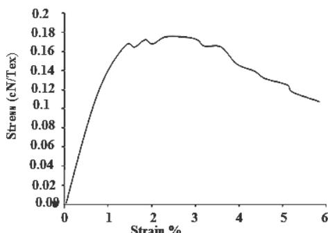
Figure 7: Stress-strain curve of fibrous assembly
