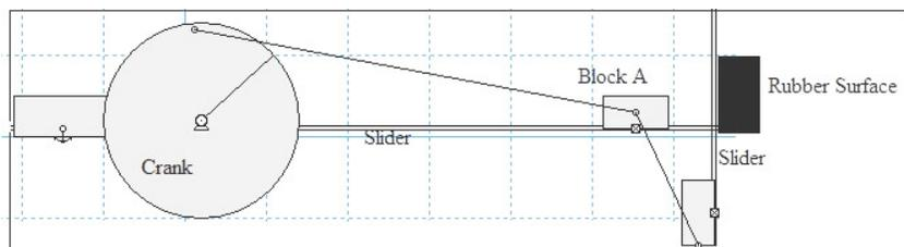
Figure 2: Schematic diagram of modified four-bar slider crank showing different parts
