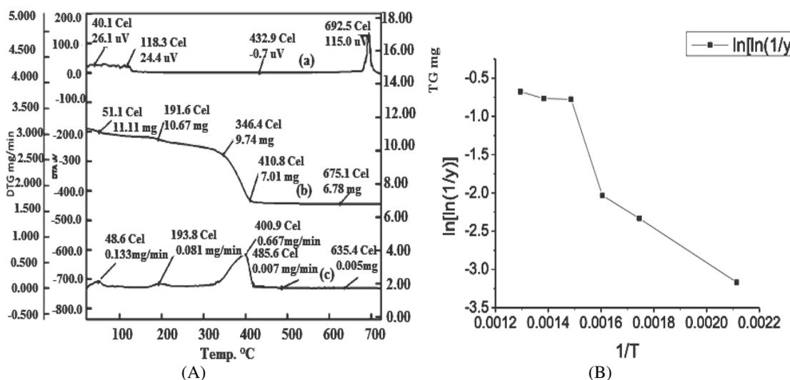
Figure 8: (A) Thermal analysis of obtained fibrous assembly: (a) DTA curve, (b) TGA curve and (c) DTG curve, and (B) graphical representation of  $\ln[\ln(1/y)]$  vs.  $1/T$  using Broido's equation
