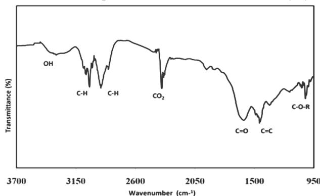
Figure 5: FTIR spectroscopy of fibrous assembly
