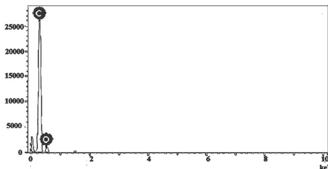
Figure 4: Elemental composition of extracted fibrous assembly by EDX
