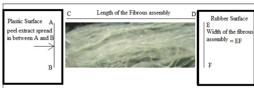
Figure 1: Diagram of manual extraction process of fibrous assembly from orange peel extract
