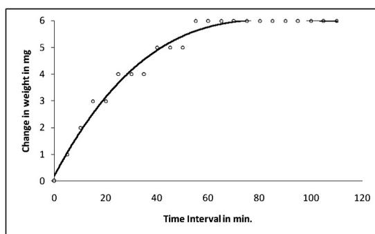
Figure 9: Weight vs. time curve depicting moisture absorbency behaviour
