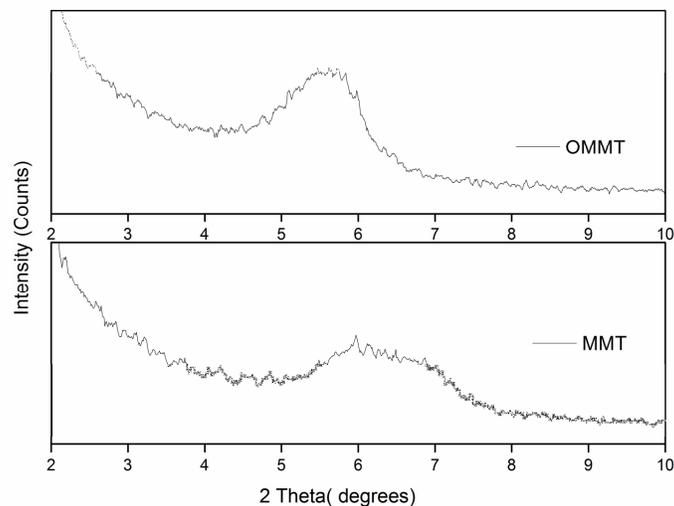
Figure 2: X-ray diffraction pattern of MMT and OMMT modified with BDDAB
