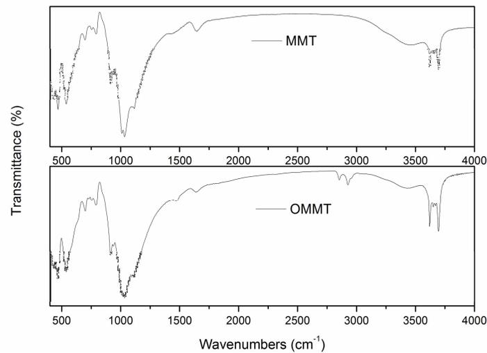
Figure 1: FTIR of MMT and OMMT modified with BDDAB
