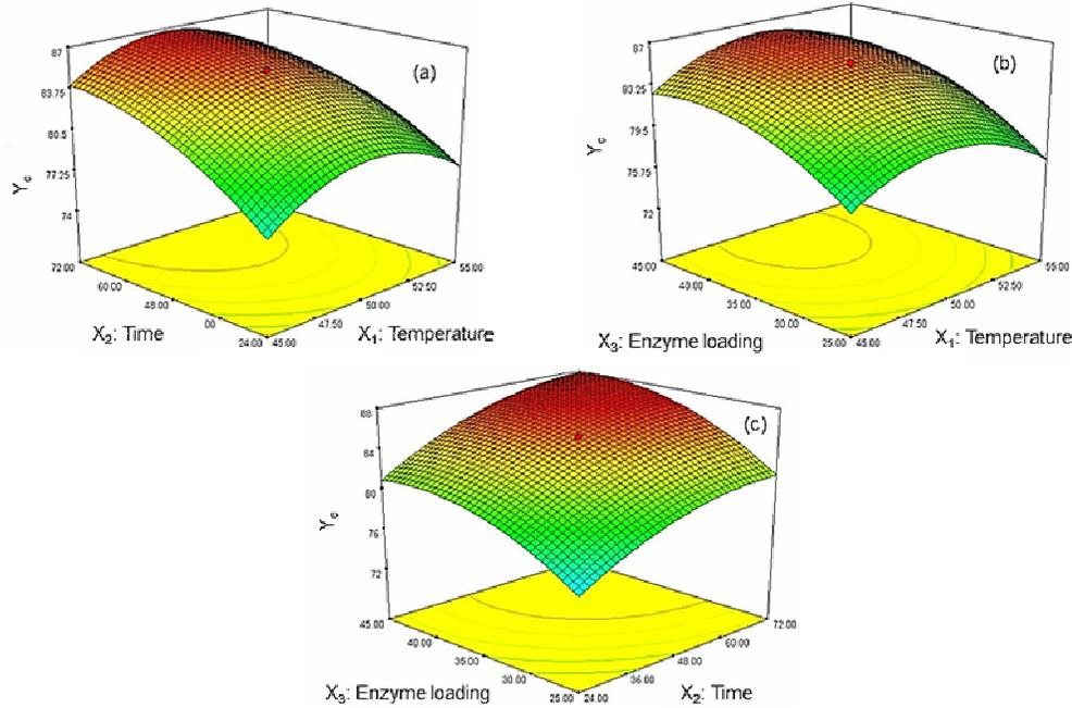
Figure 1: Contour plot of temperature and time (a), temperature and enzyme loading (b), and time and enzyme loading (c) on cellulose conversion ratio
