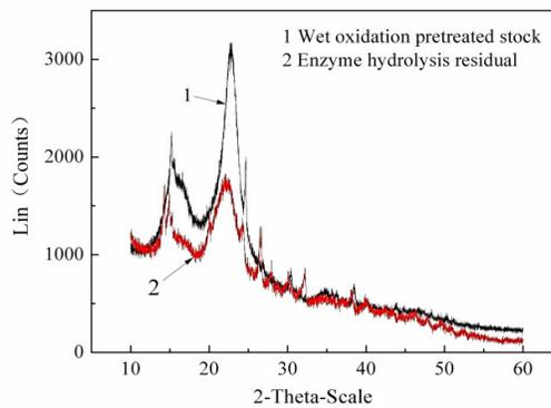
Figure 2: X-RD of WO pretreated substrate and enzymatic hydrolysis residue
