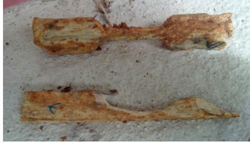
Figure 1: Typical Rubber wood degradation caused by insects under earth degradation
