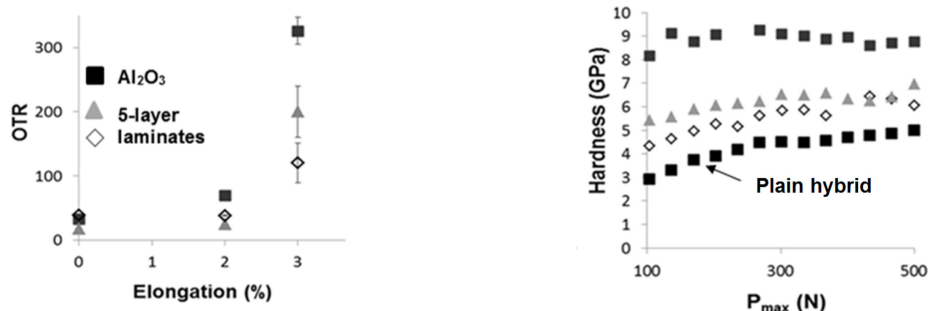
Figure 5: Effect of uniaxial straining on the oxygen barrier of PLA with different thin films (left), and hardness of the same films on silicon wafer measured by nanoindentation (right); (Further details can be found elsewhere 12,34 )
