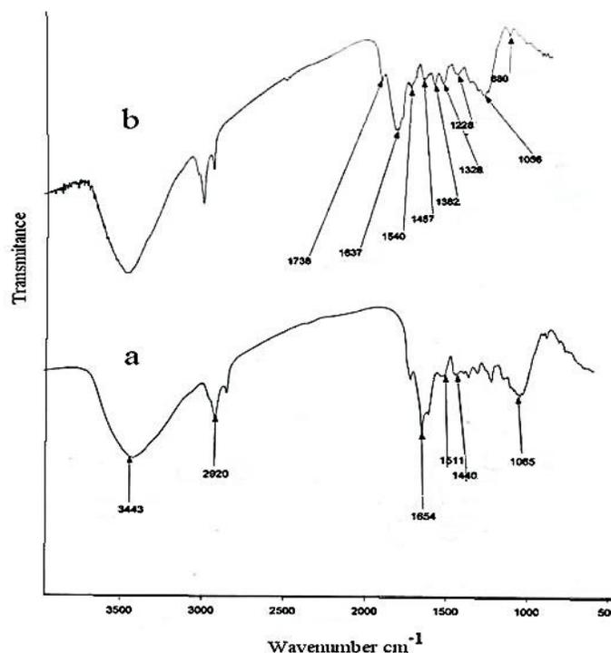
Figure 3: FTIR spectra of FTW a) before and b) after BB9 adsorption
