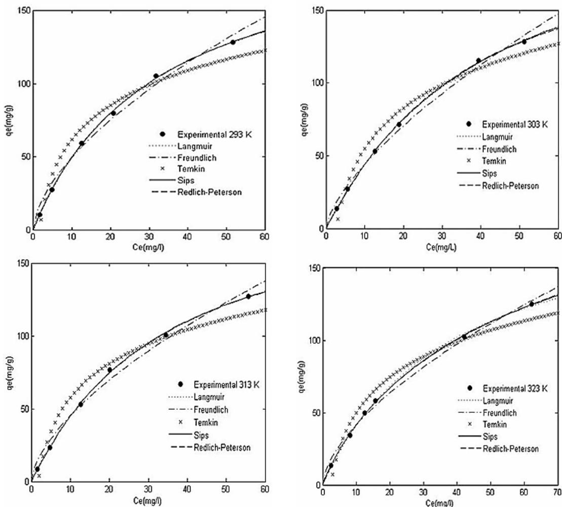
Figure 1: Isotherm plots for BB9 adsorption onto FTW at different temperatures
