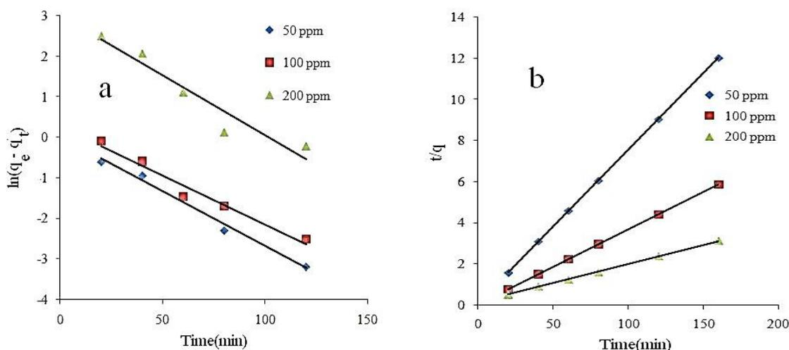
Figure 2: Kinetic models for adsorption of BB9 onto FTW; (a) pseudo-first-order and (b) pseudo-second-order rate equations
