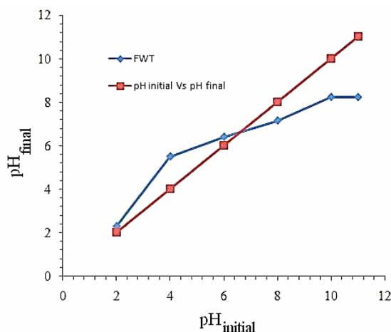
Figure 5: Plot for determination of point zero charge of FTW
